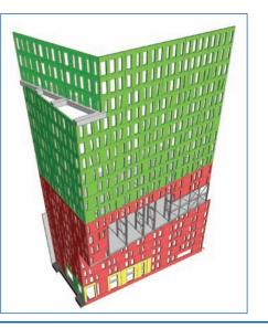
building the impression of being 'supported' by trees. 2D- and 3D-ESA-Prima Win computational models were used for the design of the prefab façades. A distinctive element is the modelling of the cantilevered prefab façade, with the steel lattice framework located behind the front, which transfers the horizontal and vertical pressure load to the rear floors.
